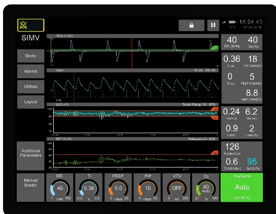
OxyGenie™ An automatic O 2 control for the SLE6000 ventilator. The SLE6000 continuously adjusts the FiO 2 to maintain a stable SpO 2 [9] .
